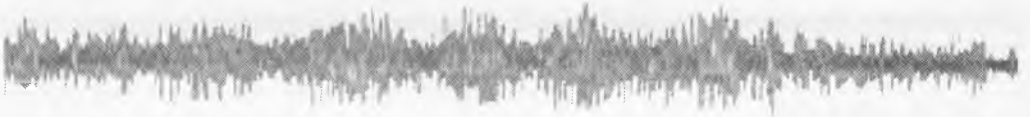
Fig. 4.27. The oscilloscope pattern of the pressure pulsations in the boundary layer of an active swimming dolphin.
