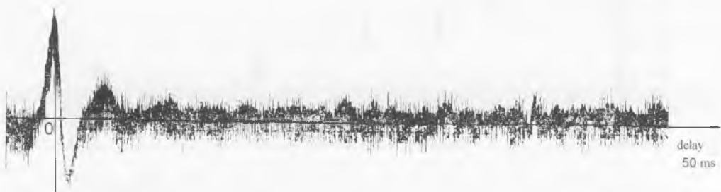
Fig. 6.41. Auto-correlation function (within the frequency band of 80 - 850 Hz) of pressure pulsations in the dolphin's boundary layer at 1.2 m from its nose.
