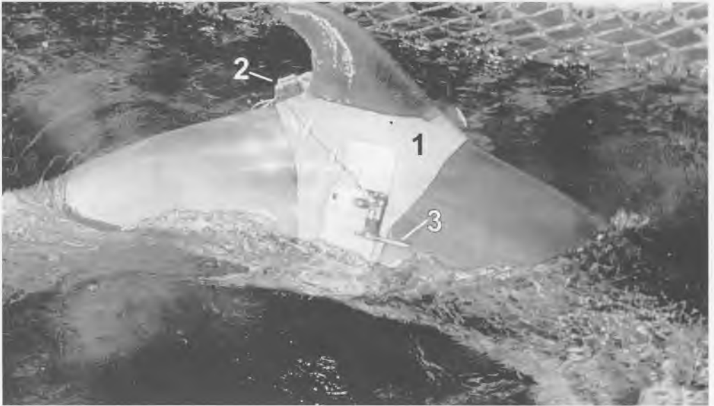
Fig. 5.56. The belt and the equipment are arranged on the dolphin. 1 – belt, 2 – equipment, 3 – pressure pulsation sensor.
