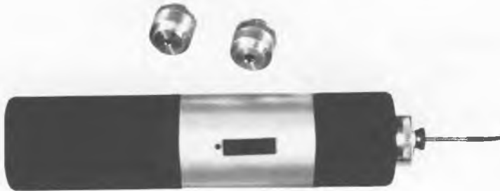
Fig. 5.22. Pistonphone with a meter installed into its calibration chamber.
