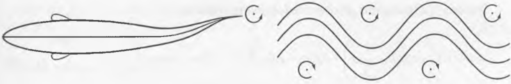
Fig. 1.22. Illustrating vortices cast off by the caudal-fin trailing edge as the fish moves to the left, and also the jet-like streamline pattern induced by those vortices. (Redrawn from Lighthill, 1969, after Karman & Burgers, 1934).
